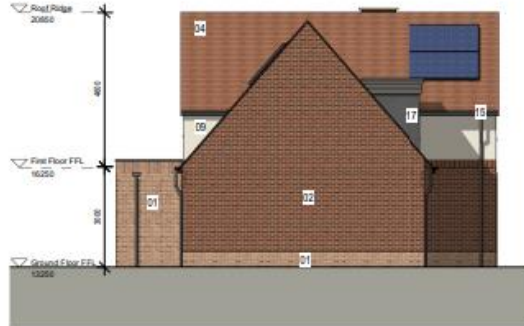
South West Elevation 1 : 100
